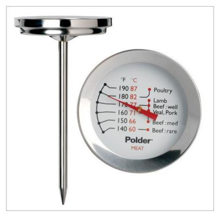
• A thermometer used to measure the internal temperature of meat, especially roasts and steaks, and other cooked foods. The degree of "doneness" of meat correlates closely with the internal temperature, so that a thermometer reading indicates when it is cooked as desired.
