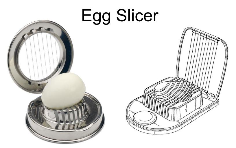
A kitchen tool with a slatted, egg-shaped hollow on the bottom and a hinged top consisting of 10 fine steel wires. When the upper portion is brought down onto a hard-cooked egg sitting in the base, it cuts the egg into even slices.
